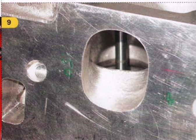
The real key to making big power is airflow. Though the stock Boss 302 heads were no slouch, these CHI 3V heads (ported by Dr. Js) offered significantly more airflow combined with an equally smaller port volume. More air through a smaller port is a surefire route to success.
