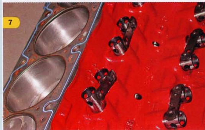
Comp Cams did supply a set of roller lifters (PN 838) for our small-block. Make sure to install these roller lifters before bolting on the cylinder heads, as the short deck height will not allow installation of the lifters after the heads are in place.
