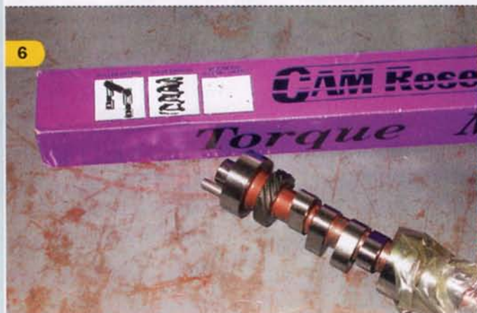
We originally tried a Comp Cams roller cam we had lying around from a previous project, but eventually settled on a dedicated stick from the Ford experts at Cam Research Corp. The Cam Research Corp grind offered a 0.721/0.724-inch lift split, a 245/249-degree duration split, and a 102-degree lobe separation angle.
