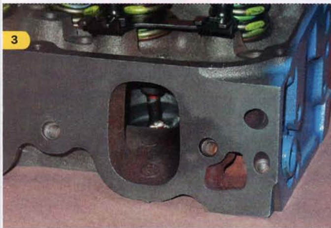
3 The stock Boss 302 heads featured huge (245cc) intake ports that offered massive airflow. In stock trim, the Boss 302 heads flow around 280 cfm—a number the Chevy guys could only dream of, even in heavily modified form.
