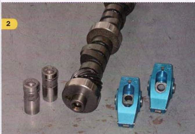
2 The stock Boss 302 was originally equipped with a solid flat-tappet cam that offered just over 0.500 lift and 228 degrees of duration at 0.050. That's mild compared to the Duntov cam used by Chevy in its 302, but the Boss more than made up for the mild cam timing with head flow.
